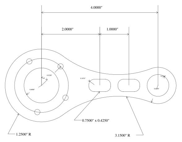
FIG. 1 - Part to be machined.
