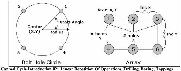
If you want to perform one operation several times in a linear pattern, simply define Position X, Y or both as incremental values. To do this, use the F1 - Abs/Inc Key. This key will toggle the Position value mode between incremental and absolute. If you define X and/or Y as incremental values, a new field will appear asking for the number of holes:
