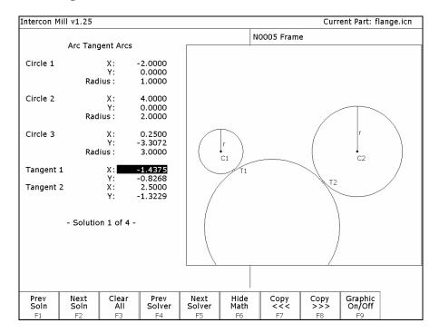
Given the center points (C1 and C2) and radii (R1 and R2) of two arcs and the radius of a third arc, find the center point of the third arc and the tangent points (T1 and T2).
