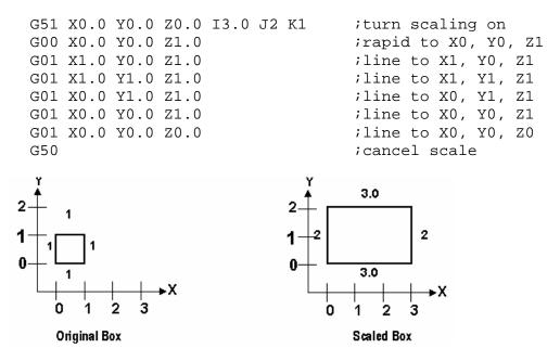
For this G51, the following program lines were scaled 3:1 in the X direction, 2:1 in the Y direction, and 1:1 in the Z direction. If no scale factor is specified, the default is 1:1 for all axes.
