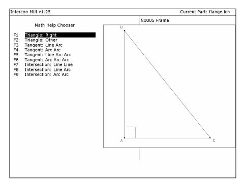
The figures on the right are a graphical representation of the highlighted solver on the left. Pressing **ENTER** key will display another menu that has various fields particular to the type of problem that is being solved. The graphic below displays the Right Triangle Calculator menu. The options that are available on the function keys are the same for every type of math help solver and perform the following operations:
