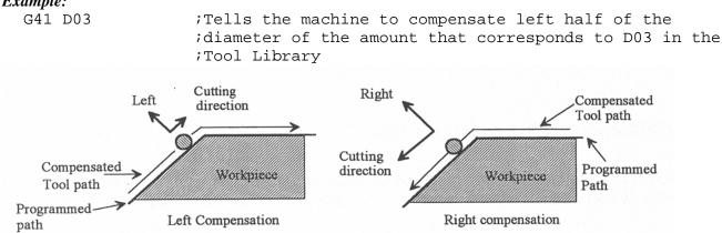
Whenever cutter compensation is applied, the following factors must be taken into account in order to obtain proper results.
