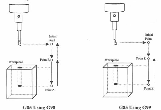
G85 is similar to G81, except that the tool is retracted with a feedrate move instead of a rapid move. G85 may be used for tapping with reversing tap heads such as the Tapmatic NCR series.
