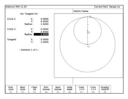
Given the center points (C1 and C2) and radii (R1 and R2) of two arcs, find the point (T) at which they are tangent.
