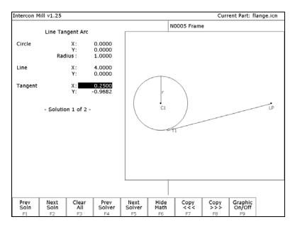
Given the center (C1) the radius of an arc, and 1 point (LP) on a line, find the lines tangent to the arc (defined by the tangent point (T1)).
