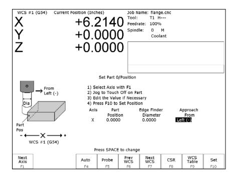
The Part Setup menu is used to set the part position or the coordinate system origin for the part.
