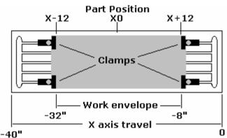
*Example:* (Machine homes to the X + switch and has 0 to -40 inches of travel in the X axis,)
