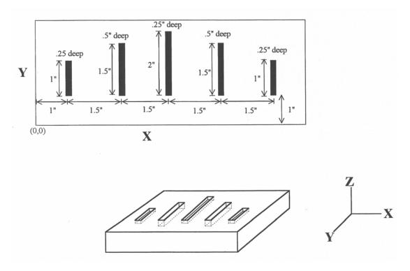
The macro variables would handle the length in the Y direction and depth in the Z direction: 00002
