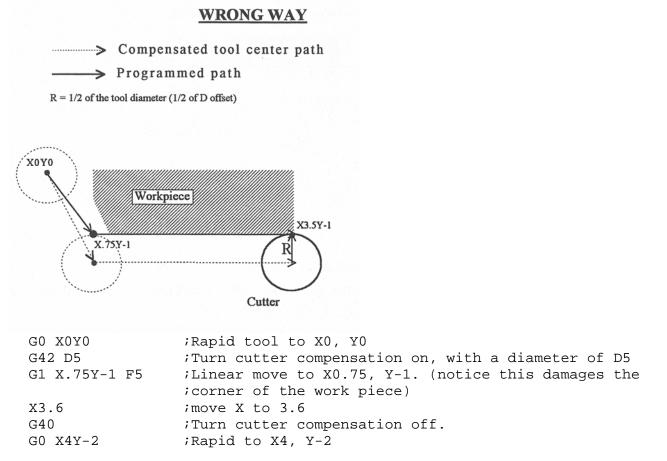
\* NOTE: This problem could have been avoided by selecting a transitional point between X0 Y0 and X.75 Y-1. A transitional point such as X-1 Y-1 would properly modify the lead-in path, keeping the cutter from damaging the corner of the workpiece. Example 3 shows the correct way of performing this operation.
