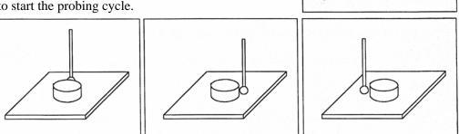
If the Z clearance you entered is too small, the probe will stop and show an error message. Correct the problem by repeating the previous steps. If the approximate diameter you entered is too small, the probe will bounce by 10 percent of its diameter across the top surface until it either finds the correct edge, the additional distance searched is equal to Parameter 16, or a travel limit is reached.
