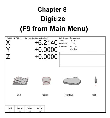
The Digitize feature of CNC10 is used to digitize a rectangular surface area (grid), an inside circular bore area (radial), or a contour. The digitizing process creates a file with M & G codes that represent the digitized surface. If the digitizing probe tip is chosen to match the milling cutter size, the digitized file can be loaded and run to produce an exact copy of the digitized part.
