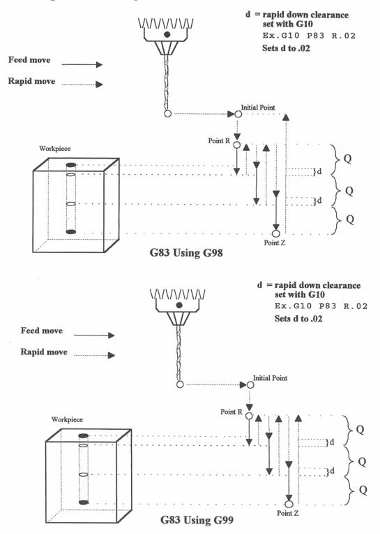
G83 is a deep hole drilling cycle. It periodically retracts the tool to the surface to clear accumulated chips, then returns to resume drilling where it left off. The retract and return are performed at the rapid rate. Because there may be chips in the bottom of the hole, the tool does not return all the way to the bottom at the rapid rate. Instead it slows to feedrate a short distance above the bottom. This clearance distance is selected by setting Parameter 83 with G10 (see example below).
