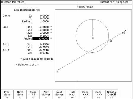
Given the center (C1) and radius (R) of an arc, 1 point (P1) and either a second point (P2) or one coordinate (P2 X or Y) and the angle from horizontal, find the intersection point(s) (I1 and I2).
