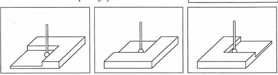
At the end of the probing cycle, the probe will be positioned above the corner at the Z clearance level entered. Press **ESC** to return to the Set Part 0/ Position screen or digitize screen.
