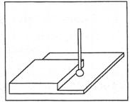
Once the probe has completed its search, it will be positioned above the corner at the Z clearance you specified. Press **ESC** to return to the Set Part 0/ Position screen or digitize screen.
