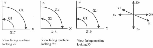
\* NOTE: When using G18, the G2 command moves in a counterclockwise direction in the XZ plane.
