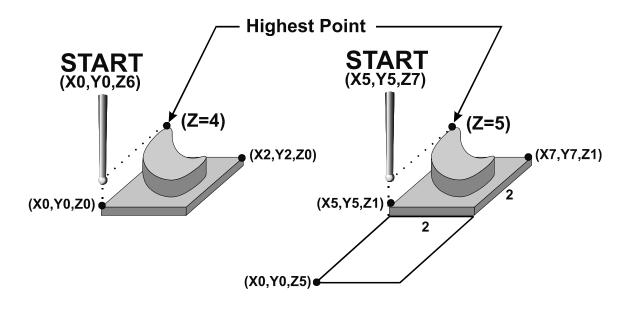
3. A good technique for calculating Z maximum depth is to touch off the lowest surface of the part to be digitized and set the part zero's Z value to Z0. Then jog the probe tip to a point higher than the highest surface of the part to be digitized. Note the displacement in the Z-axis. Again, set this Z height to Z0 and use the noted displacement for the Z maximum depth.
