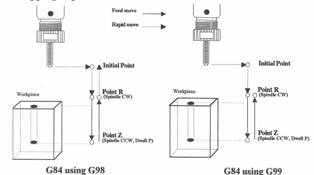
G84 performs right-hand tapping using a floating tap head. The spindle speed and feedrate should be set and the spindle started in the CW direction before issuing G84. By default G84 uses M4 to select spindle CCW (at the bottom of the hole) and M3 to re-select spindle CW (after backing out of the hole). Alternate M functions may be specified by setting parameters 74 (for CCW) and 84 (for CW). See G10 for examples.
