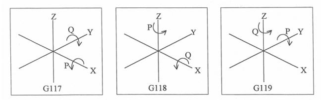
For the G117 plane, the "first axis" is X and the "second axis" is Y.
