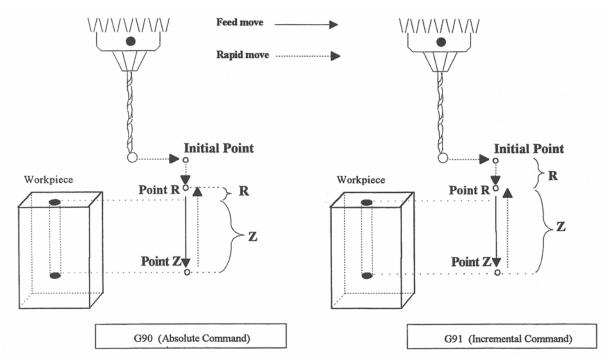
Figure 2: Canned Cycle Absolute and Incremental modes
