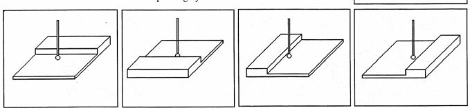
Once the probing cycle is complete, the probe will move away from the surface by the amount entered in Parameter 13 (Recovery Distance). The dimension where it found the surface will be shown on the control. Press **ESC** to return to the Set Part 0/ Position screen or digitize screen.
