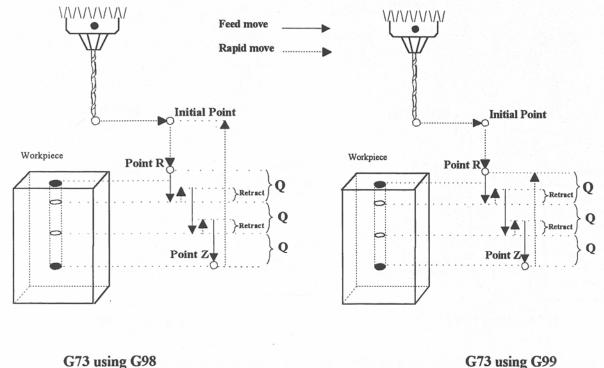
G73 is the peck drilling cycle. The hole is drilled in a series of moves: down a distance Q at a given feedrate, up the retract distance at the rapid rate, and then down again at the given feedrate. The retract amount is set with G10 as shown in the example below.
