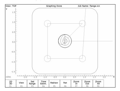
The display will consist of arcs and/or lines that make up the tool path followed. Rapid (G0) moves will appear in Red, linear (G1) and arc (G2, G3) moves will be Yellow, and compensated pass will appear in grey. Canned cycle operations (except the facing cycle) will also display a gray.
