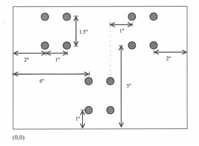
Suppose that a drilling pattern of 4 holes is needed in 3 different locations:
