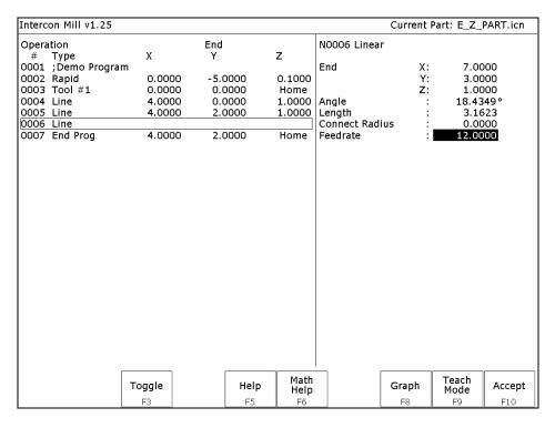
The numbers in the different fields on the screen correspond to the following Linear Mill example shown here graphically:
