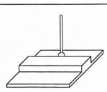
If the Z clearance you entered is too small, the probe will stop and show an error message. Correct the problem by repeating the previous steps. If the approximate width you entered is too small, the probe will bounce by 10 percent of its width across the top surface until it either finds the correct edge, the additional distance searched is equal to Parameter 16, or a travel limit is reached.
