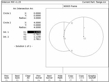
Given the center points (C1 and C2) and the radii (R1 and R2) of two arcs, find the intersection point(s) (I1 and I2) of the arcs.
