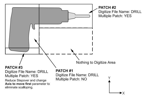
The drill shown in the previous example is L-shaped. Therefore, it can be digitized faster and more efficiently using three rectangular patches than digitizing the complete area with a single patch.
