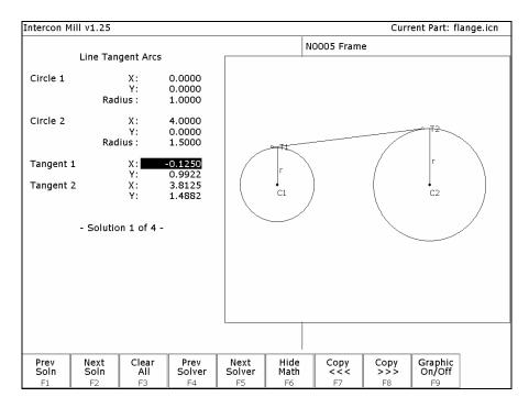
Given the center points (C1 and C2) and radii (R1 and R2) of two arcs, find the lines (defined by T1 - T2) tangent to both arcs.
