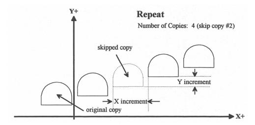
Increment: Specifies the X and Y distances between the start points of each copy of the contour.
